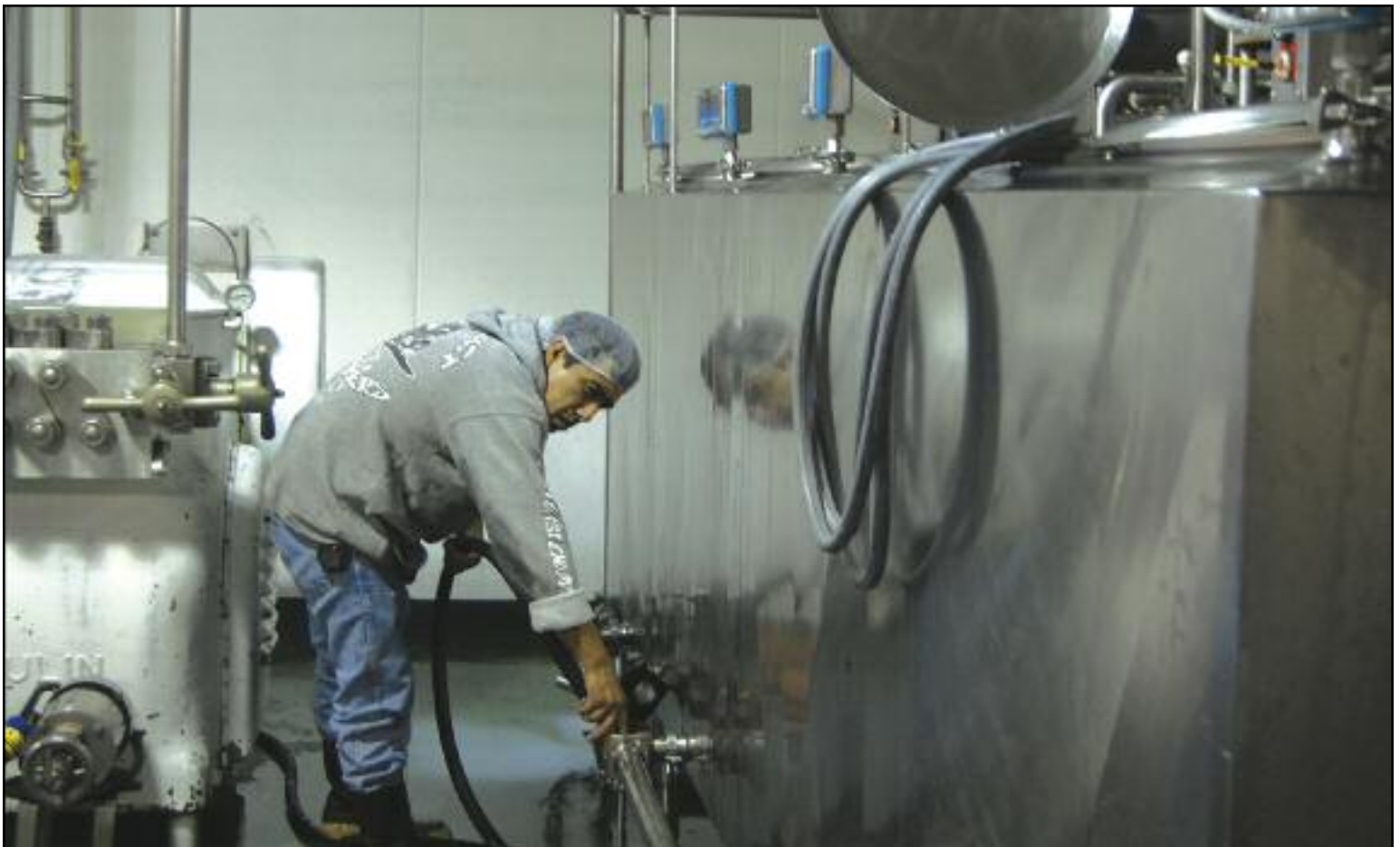
A Sparkman's employee cleans the storage tank after milk production is finished for the day. The pipes are part of the system in which fats and solids initially are removed from the milk and then reinserted to make different types of milk and chocolate milk. Excess fats and solids are used in the production of cream and butter. Photo by Alan Mauldin
